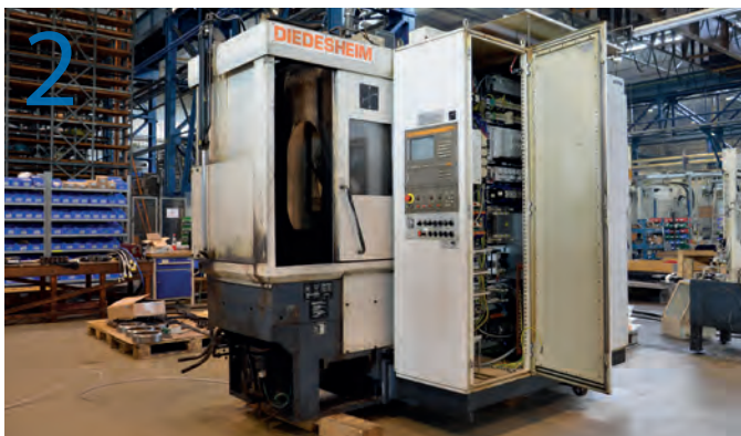
3 lathes for gearwheel manufacturing / Maker: DIEDESHEIM
